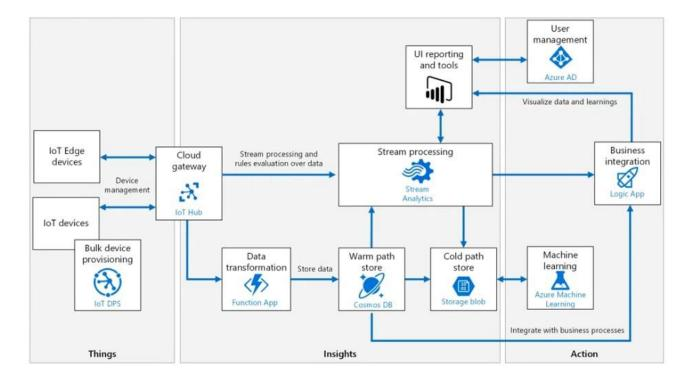
**IOT Edge devices:** Devices cannot be constantly connected to the cloud in this case IOT edge devices contian some processing analysis logic within it. So that there is no constant dependency for the cloud.
