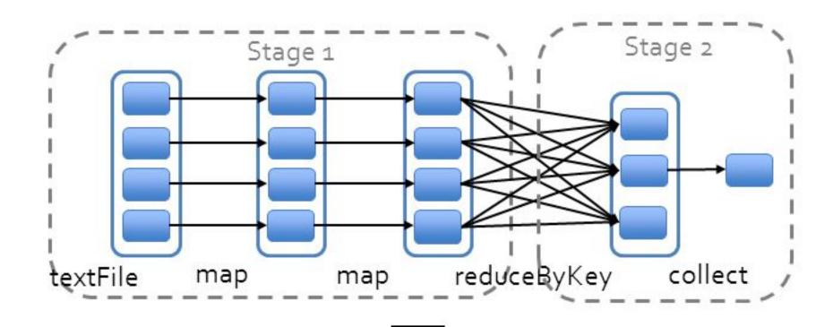
read HDFS split apply both maps partial reduce write shuffle data
